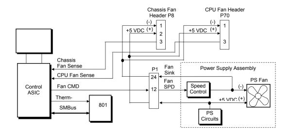
Figure 4-12. Desktop/Configurable Minitower Fan Control Block Diagram
